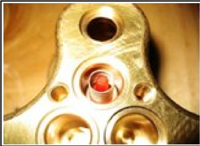
Pic. F21: Pressure valves
